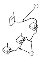
Field wire 1 is run to first detector in Hot-Loop group. Other lengths of field wire 2 connect other detectors with each other in "Parallel".
