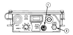
To erase memory, press TEST RESET button (2) on receiver.
